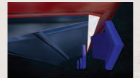
Reverse chines along hull sides to deflect spray
